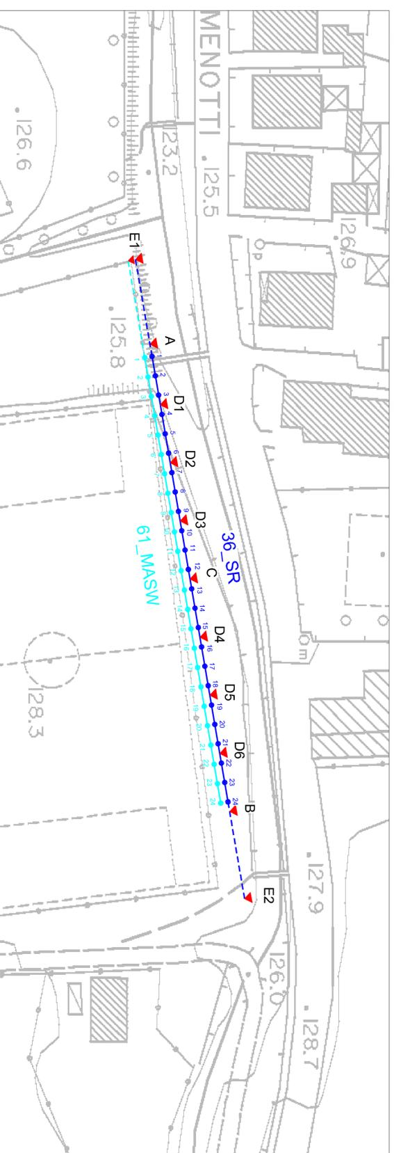
50\_SR PROVA SISMICA A RIFRAZIONE ONDE P E ONDE SH E 62\_MASW - SCALA 1:500
